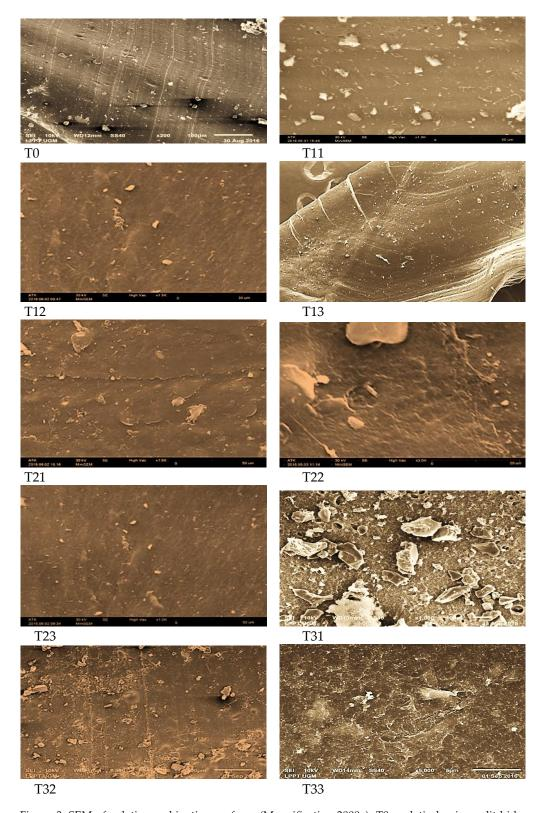
Figure 3. SEM of gelatin combination surfaces (Magnification 2000x). T0= gelatin bovine split hide; T11, T12, T13= gelatin bovine split hide: SPI = 90: 10 + TG ase enzyme 10, 20, 30 U; T21, T22, T23= gelatin bovine split hide: SPI = 80: 20 + TG ase enzyme 10, 20, 30 U; T31, T32, T33= gelatin bovine split hide: SPI = 70:30 + TG ase enzyme 10, 20, 30 U.
