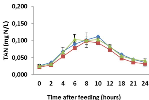
Figure 6. Total ammonia nitrogen (TAN) of yellow tail *Seriola quinqueradiata* in the outlet water of seaweed tanks at different flow rates (0.5 L min<sup>-1</sup> (◆), 1 L min<sup>-1</sup> (■) and 1.5 L min<sup>-1</sup> (▲)) in day 20.
