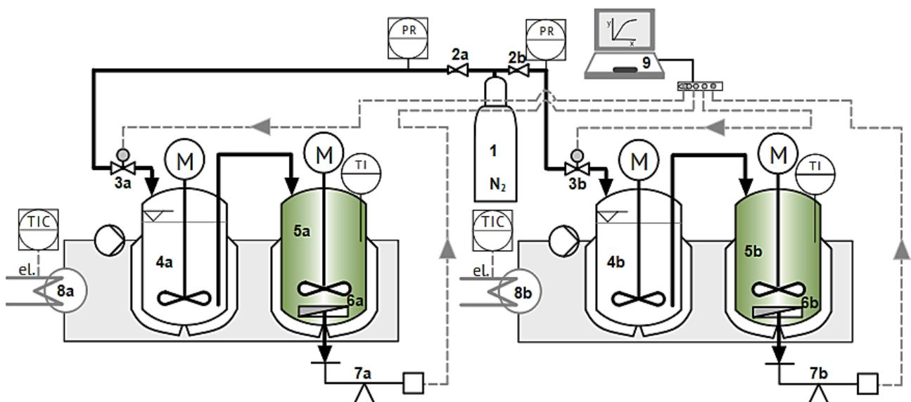
Note: 1= Nitrogen (N<sub>2</sub>), 2= pressure reducer, 3= proportional pressure regulator, 4= substrate tank, 5= stirred tank reactor, 6= UF membrane, 7= analytical balance, 8= water bath, 9= PC. M: motor, PR= pressure register, TIC= temperature indicating controller, TI= temperature indicator, el.= electricity
