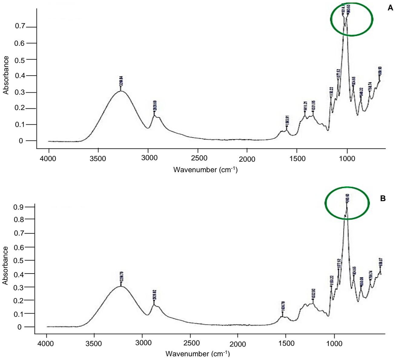
Figure 4. Fourier transform infrared spectroscopy (FTIR) chromatogram of bioplastics control (A) and bioplastic fortified with FSME (B)
