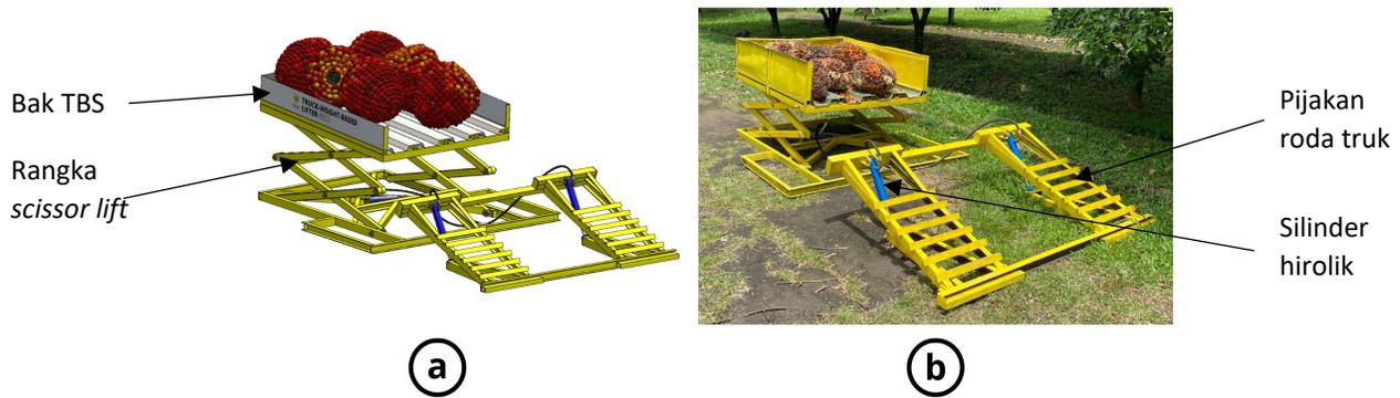
**Gambar 5.** *Truck-Weight-Based FFB Lifter*: (a) model, (b) aktual.
