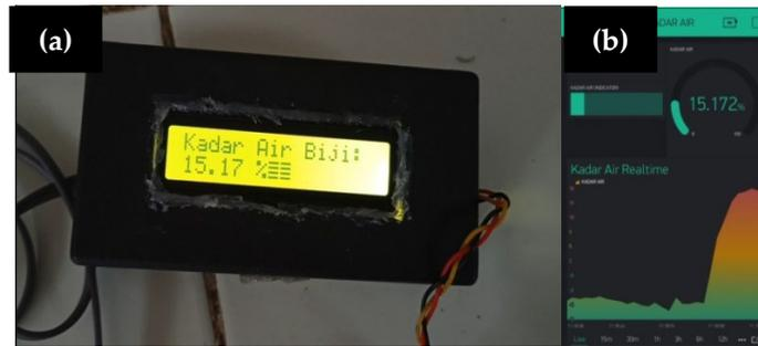
**Figure 5.** Test Results on (a) LCD and (b) Blynk Application
