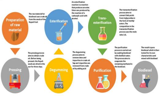
Figure 1. Biodiesel production process flow chart
