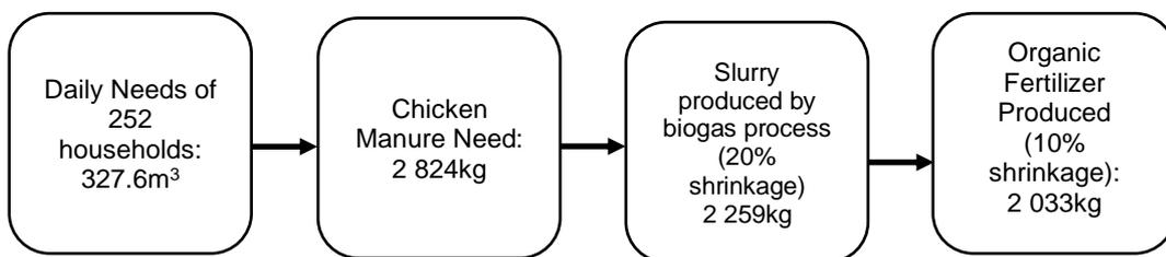
Figure 2 The process of chicken manure into biogas
