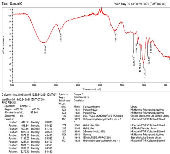
Figure 6 FTIR in sample C
