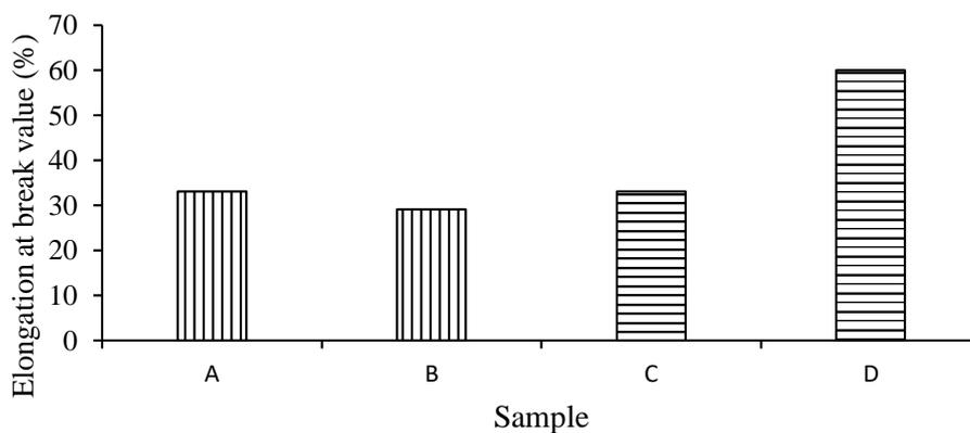
Figure 2 Elongation at break of bioplastic
