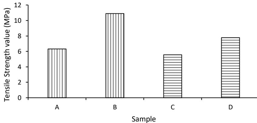
Figure 1 Tensile strength of bioplastic product
