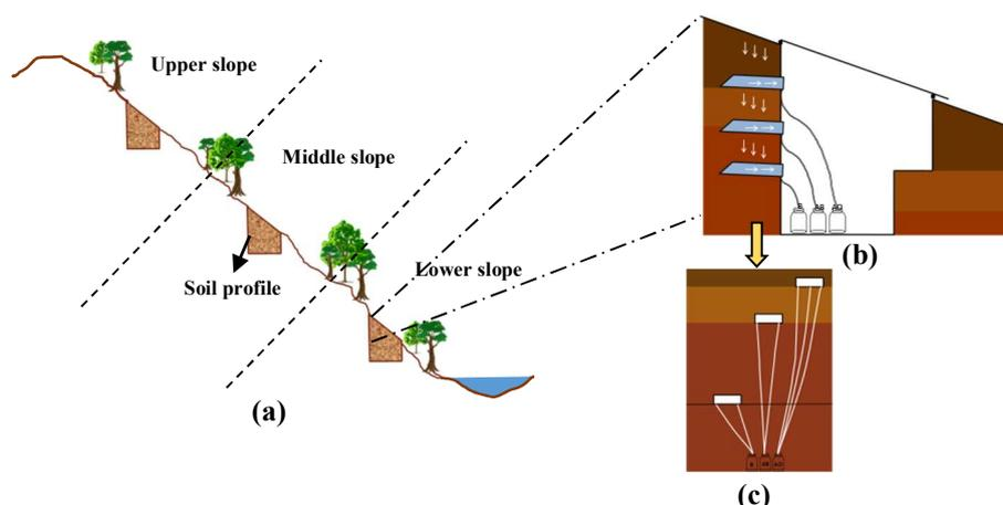
Figure 1 (a) Position of soil profiles, (b) Design of lysimeters instalation (side view), (c) Lysimeter instalation (front view).
