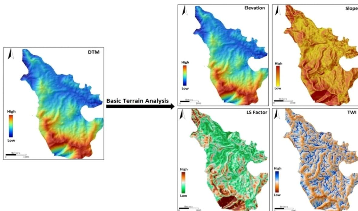
Figure 4 Process of map derivation for selected terrain parameters.
