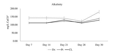
Figure 2. Fluctuations in the alkalinity concentration in the biofloc system aquaculture water over 30 days with different carbon sources.
