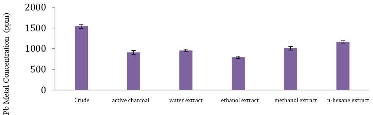
Figure 2. Lead (Pb) Metal Absorption of the Extracts
